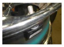
To avoid damaging sensors when demounting tires, do not break the bead within 45 of either side of sensor assembly locations. Be careful not to damage sensors when mounting tires as well. Sensors are not repairable and require replacement if damaged or when their battery is completely drained. It is recommended that the sensor be carefully "dropped into the tire" prior to demounting to avoid damage.
