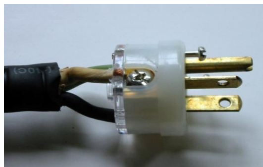
Picture 1: white neutral wire under silver screw
