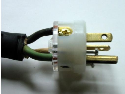
Picture 2: black "hot" wire under screw
