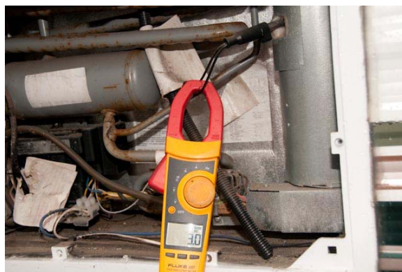
Measuring amp draw through the electric element on the refrigerator
