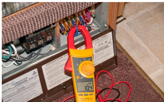
Measuring direct current with the furnace running.
