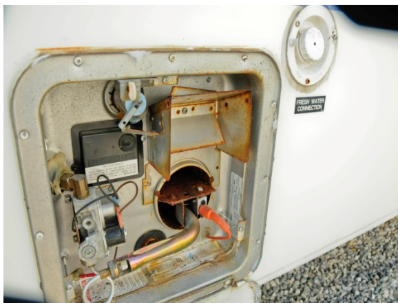
Water heater with cover removed from the burner tube for cleaning
