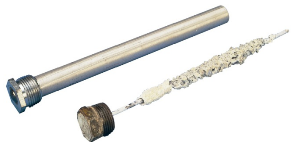
A new anode rod and one that needs replacing
